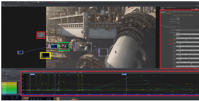
Figure 3: Screen capture of the TouchDesigner workflow: red – Animation COMP-related modules; green – StreamDiffusion node; yellow – ControlNet
